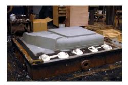
From these files, foam molds are produced using a computerised mill. In the image above you see the interior of the SASA-172 and in the image above you see one of the doors.
