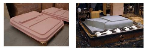
From these files, foam molds are produced using a computerised mill. In the image above you see the interior of the SASA-172 and in the image above you see one of the doors.
