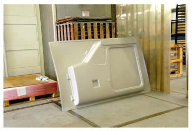
Finally, one of the molds for one side of the fuselage. As you can see, these molds are very big.
